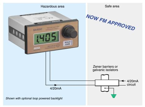
The BA405C is an intrinsically safe panel mounting manual set point station that enables the current flowing in a 4/20mA loop to be manually adjusted from within a hazardous area. The instrument is loop powered and contains a 3½ digit display which may be calibrated to show the 4/20mA current in engineering units.
