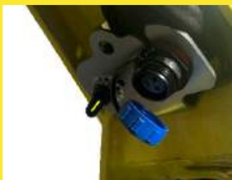
Under the seat , you will find the charger connector. Remove the connector cap.
