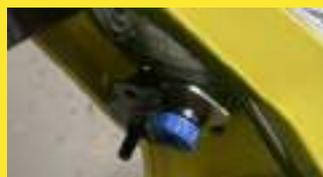
Remember to put again the blue tap on, when the battery is fully charged.
