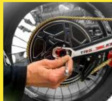
Unscrew the chain tensioner with a 8mm wrench by pushing the chain tensioner. Perform the same operation on the other side of the swingarm. Fix the locknuts and screw the wheel axle. Check that the pinion and crown screws are correctly screwed.
