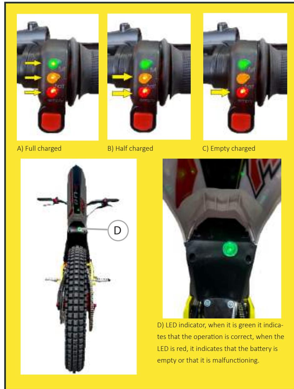
D) LED indicator, when it is green it indicates that the operation is correct, when the LED is red, it indicates that the battery is empty or that it is malfunctioning.
