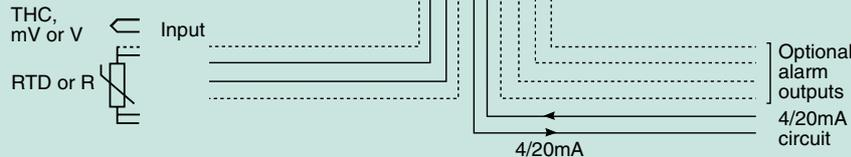
The new BA678C is a second generation panel mounting, loop powered indicating temperature transmitter which replaces the BA578C. It provides an accurate local digital temperature display, plus a 4/20mA output, which may be scaled to represent any temperature range. Although incorporating new facilities such as HART® digital communication, diagnostics and a robust enclosure with a IP66 front panel, the BA678C remains electrically compatible with the earlier model.
