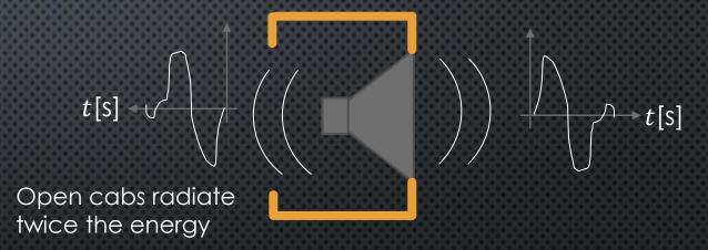
The 'trapped' air will have an impact on the resulting 'effective' speaker stiffness, especially for a small, closed, cabinet
