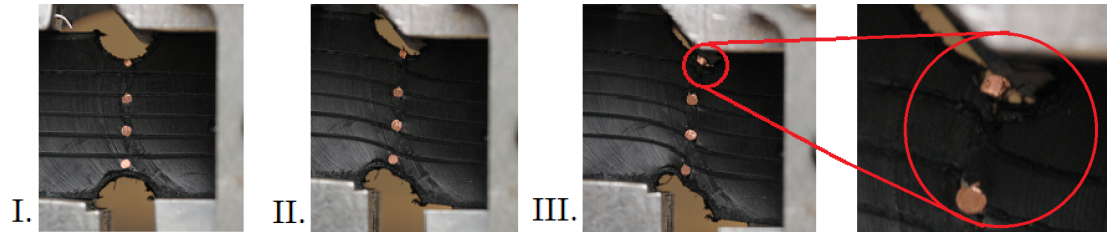
Figure 4.9: Shear experiment on specimen from a successful fusion.
