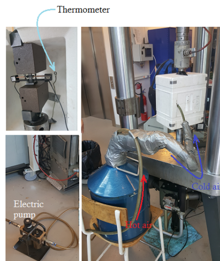
Figure 4.3: Setup for the tensile test in temperature of 10 °C.
