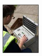
will also require no maintenance for at least five years. With a typical five year battery life, LCD screen with backlight and simple push button interface, the SoundSens "i" can be used at any time of the day or night.
