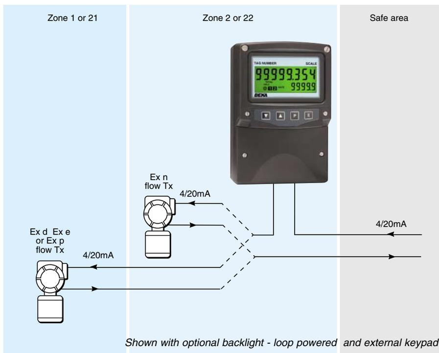
The BA354NE loop powered 4/20mA rate totaliser is a third generation field mounting instrument that is electrically and mechanically compatible with the earlier BA354ND, but it has a larger display, extended operating temperature and additional features such as a lineariser and bi-directional flow capabilities. Like its predecessor the BA354NE is housed in a robust IP66 GRP enclosure with a separate terminal compartment.
