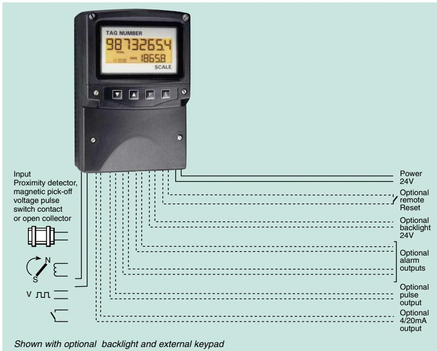
The **BA534D** is an externally powered rate totaliser with separate rate and total displays which will operate from a switch contact, voltage pulse, magnetic pick-off, open collector or a proximity detector input. A novel adaptive measuring technique plus an adjustable digital filter ensure that optimum rate display stability and step response can be achieved over a wide input frequency range.
