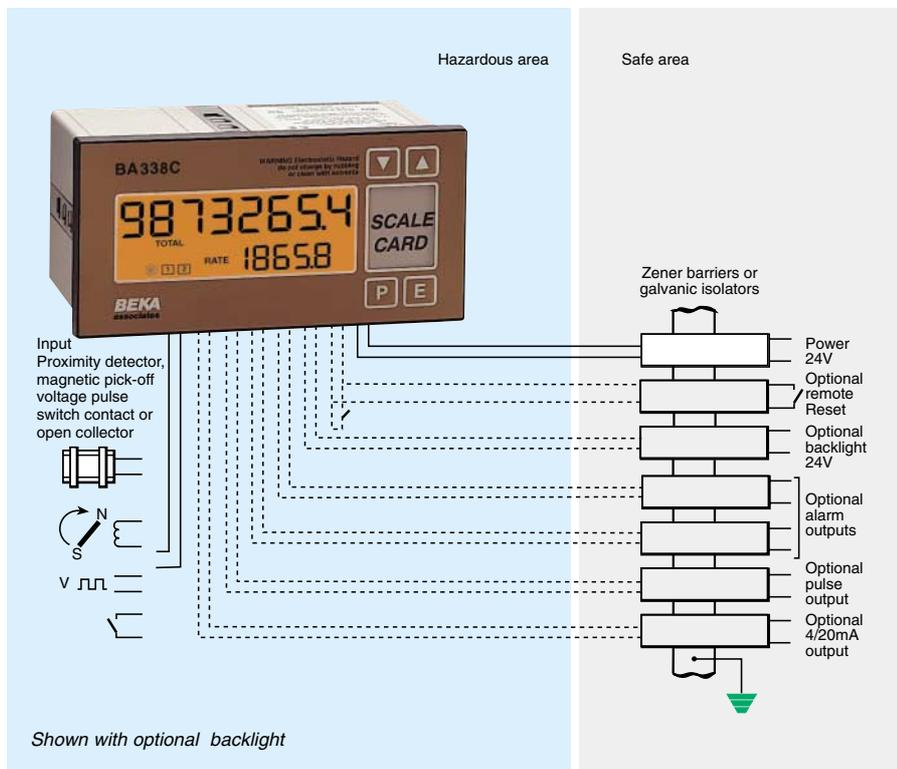
The **BA338C** is an externally powered, intrinsically safe rate totaliser with separate rate and total displays which will operate from a switch contact, voltage pulse, magnetic pick-off, open collector or a proximity detector input. A novel adaptive measuring technique plus an adjustable digital filter ensure that optimum rate display stability and step response can be achieved over a wide input frequency range.
