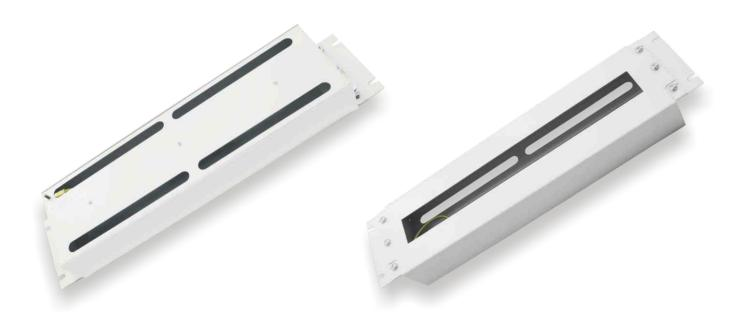
Universal 19" or 21' enclosure for modular devices. 1.5 mm thick sheet powder painted in light grey (RAL 7035), DIN rail included, housing with 402.5 x 45.5 mm opening.
