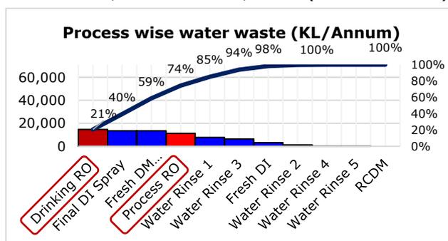
Water coming out from sub-processes like Drinking RO plant water, Process RO plant, Final DI spray, Water rinse cycles etc. is going in waste. So, scope is there for 3R (Reduce, Recycle and Reuse) in these 8 sub processes. But the challenge is to contain water conductivity within 2 micro-siemens ( $\mu\text{S}$ )/cm
