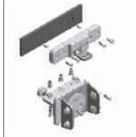
In order that the frame bracket support spindle can be used on the transom/mulliom, the transom-mulliom construction must have a minimum depth of 100mm. Without support spindle, only a load of approx. 1500N is possible.
