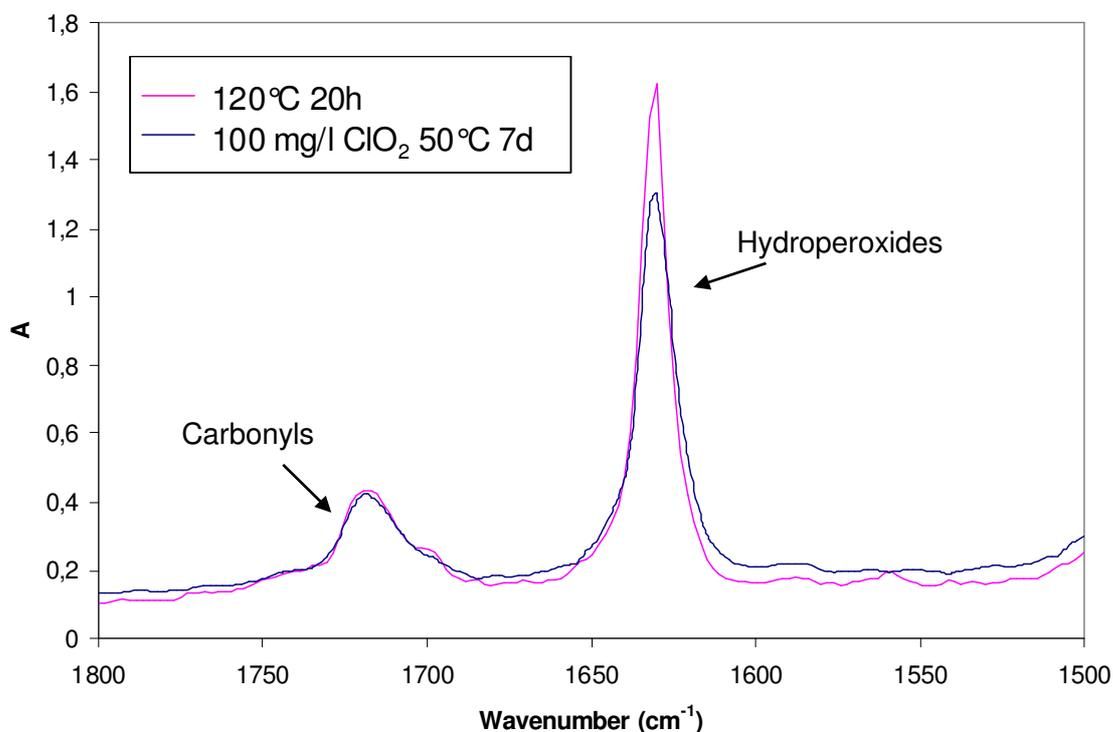
**Figure 1.** Unstabilised UHMWPE exposed in air at 120°C for 20 hours and to 100 mg/l ClO<sub>2</sub> for 7 days at 50°C. The reaction products are almost identical (carbonyls at 1720 cm<sup>-1</sup> and hydroperoxides after NO reaction at 1630 cm<sup>-1</sup>).
